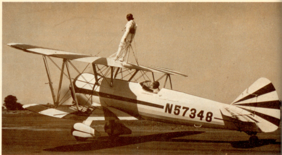
This former Army PT-17 has been fitted with a 450 h.p. Wasp Jr. engine and dressed up for air show work. Sunburst paint job for upper surfaces is almost a mandatory uniform for exhibition ships.
